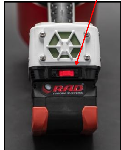
Figure 2.3.1-1: Battery Release and Lock Out
