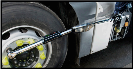
An DBW1000 breaking over at set torque.
