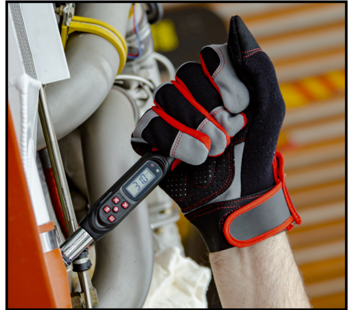
EDWM020 used to tighten motor compartment bolts on Cirrus SR22 aircraft.
