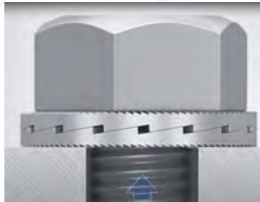
HEICO-LOCK® prevents self-loosening.
