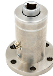
Digital Torque Tester DTT1000 Range: 100 – 1.000 Nm
