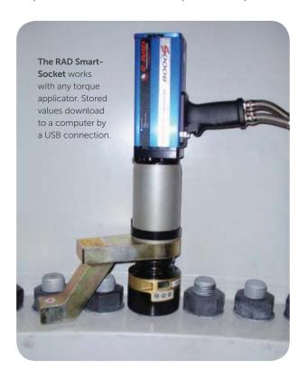
in a joint. This ensures the fastener is adequately tight and will not come loose under general working conditions. This torque is typically applied using a torque wrench, impact wrench, hydraulic torque wrench, or pneumatic torque tool, which has been calibrated and certified to ensure accuracy and traceability. Accurate and repeatable applications of the required torque are essential to guarantee the joint's integrity.
